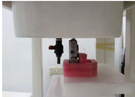
Fig.8 EUT Left side to flat phantom
