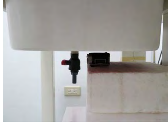
Fig.3 EUT Front side to flat phantom
