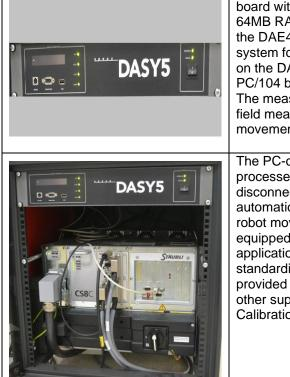
The DASY5 measurement server is based on a PC/104 CPU board with a 166MHz low-power Pentium, 32MB chip disk and 64MB RAM. The necessary circuits for communication with either the DAE4 electronic box as well as the 16-bit AD-converter system for optical detection and digital I/O interface are contained on the DASY5 I/O-board, which is directly connected to the PC/104 bus of the CPU board. The measurement server performs all real-time data evaluation for
