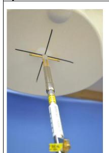
Construction: Symmetrical dipole with I/4 balun Enables
