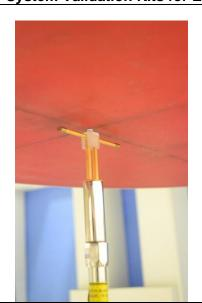
Construction: Symmetrical dipole with I/4 balun Enables
