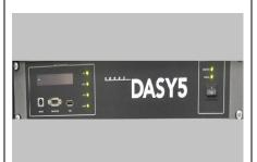
The DASY5 measurement server is based on a PC/104 CPU board with a 166MHz low-power Pentium, 32MB chip disk and 64MB RAM. The necessary circuits for communication with either the DAE4 electronic box as well as the 16-bit AD-converter system for optical detection and digital I/O interface are contained on the DASY5 I/O-board, which is directly connected to the PC/104 bus of the CPU board.
