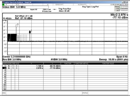
Marker 1: - End of Burst : 1.186 s Marker 2: - End of Transmission : 2.976 s
