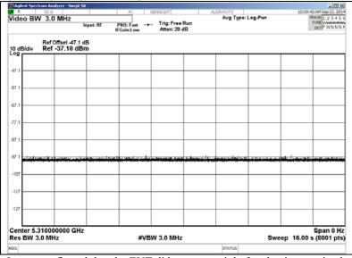
It was confirmed that the EUT did not transmit before having received appropriate control signals from a Master Device.
