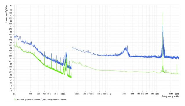
Spurious emissions from 9 kHz to 30 MHz (operation mode reading TAG continuously):
