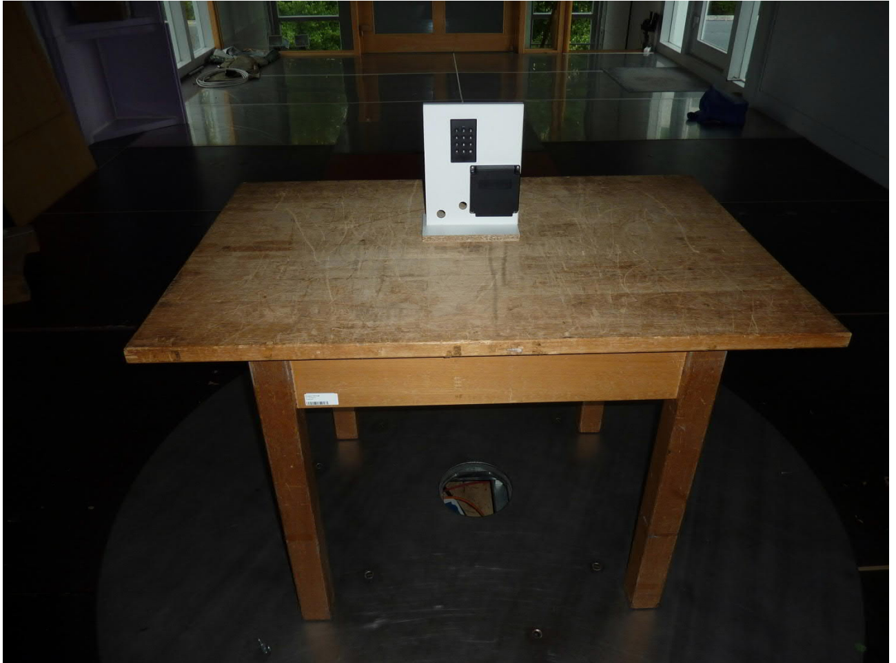
Keypad TA03 with lock M610 Test setup –final measurement
