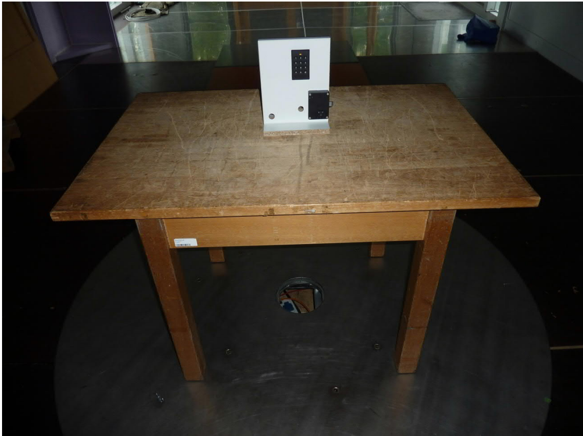
Keypad TA03 with lock M410 Test setup –final measurement
