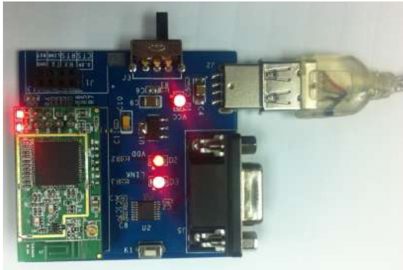
Figure 3-1 connection between with serial adapter board and UART-WIFI module
