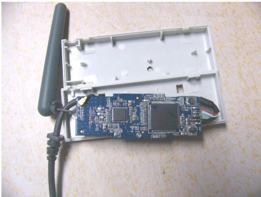
Main & RF board component side
