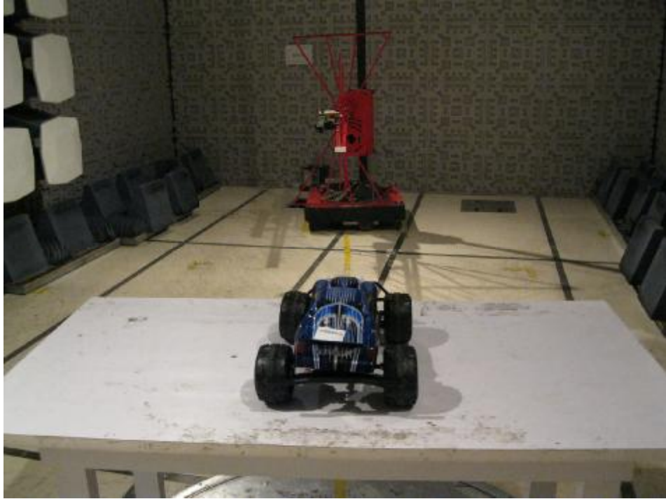
TEST SETUP OF RADIATED EMISSION
