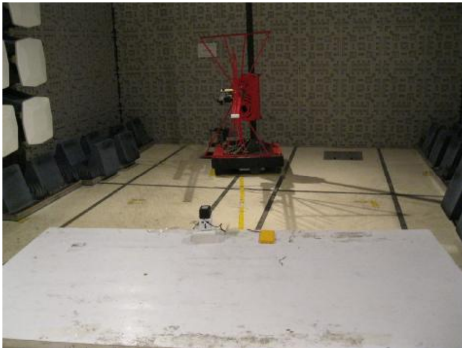
TEST SETUP OF RADIATED EMISSION
