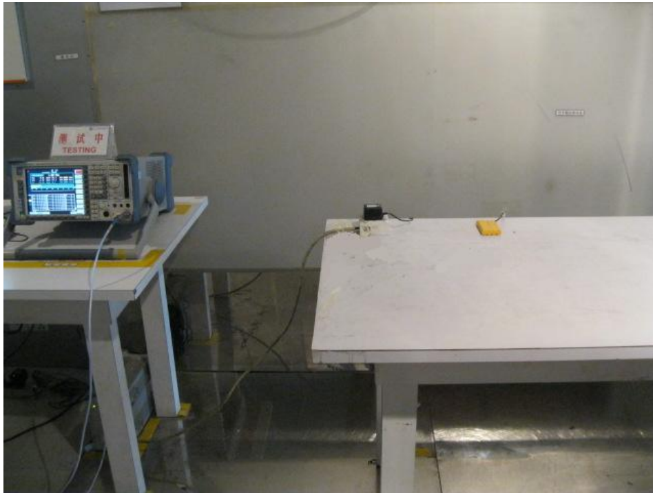
TEST SETUP OF CONDUCTED EMISSION
