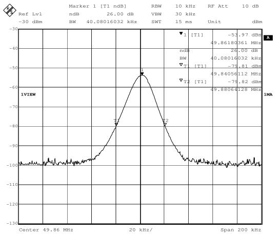
The 26dB down bandwidth lower edge is: 49.84056MHz The 26dB down bandwidth upper edge is: 49.88064MHz
