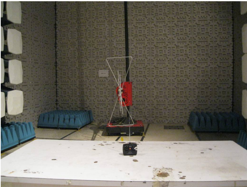
TEST SETUP OF RADIATED EMISSION (30MHz-1GHz)
