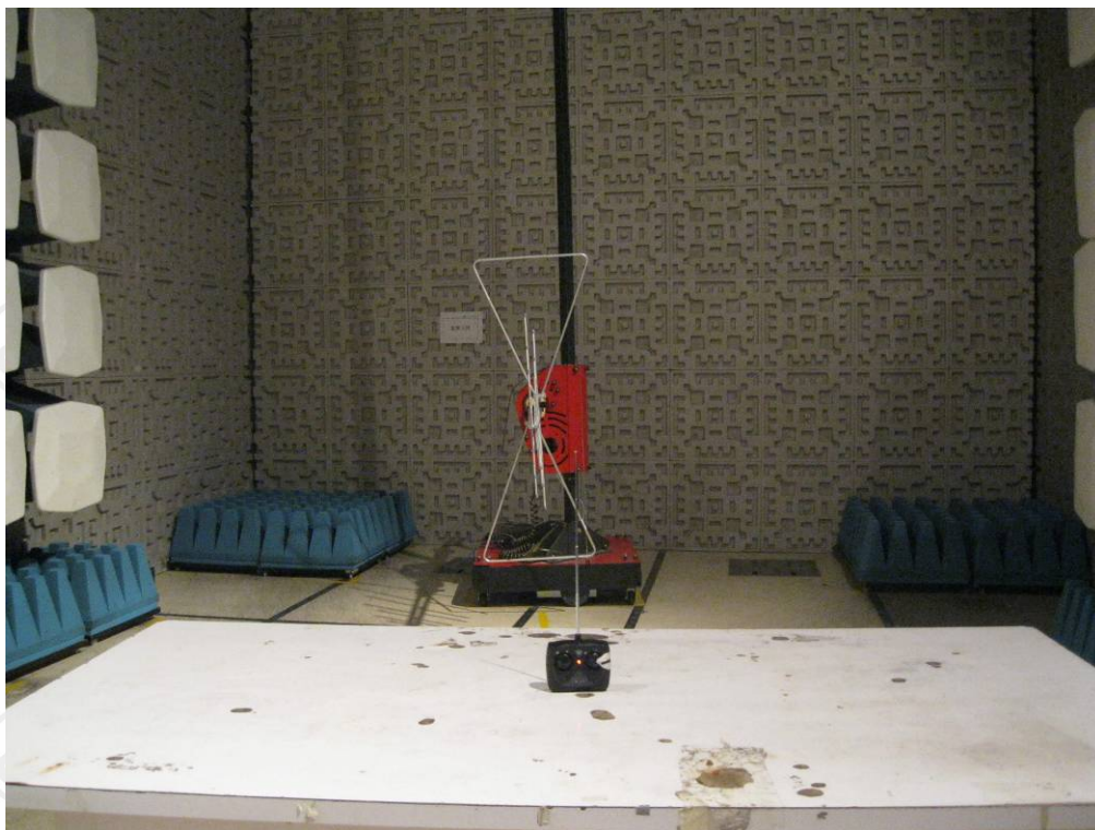
TEST SETUP OF RADIATED EMISSION (30MHz-1GHz)
