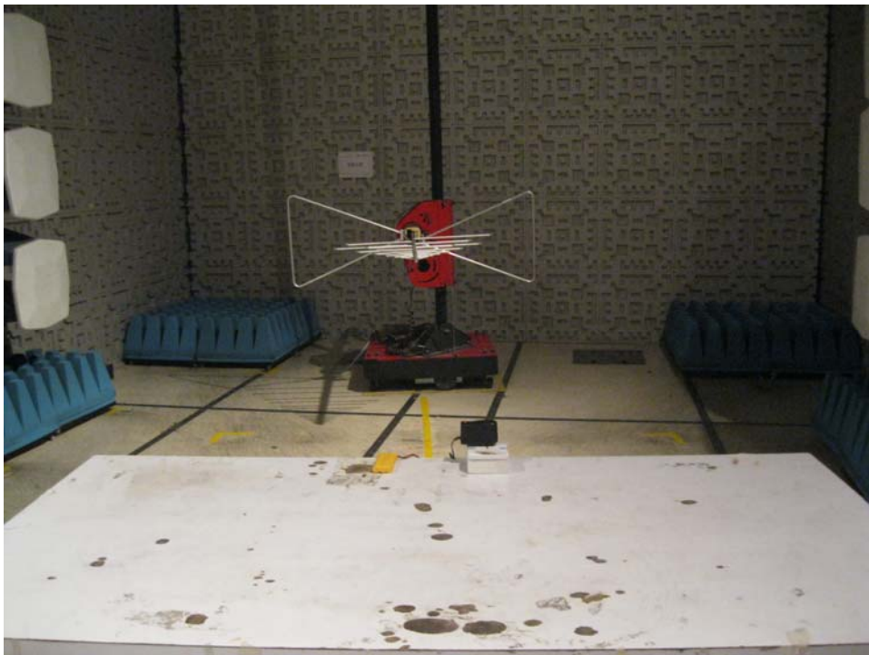
RADIATED EMISSION TEST SETUP-2
