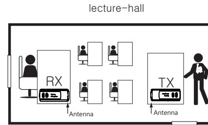
※ Aligning of wireless transmitter/receiver antennas facing each other gains better receiving sensitivity.
