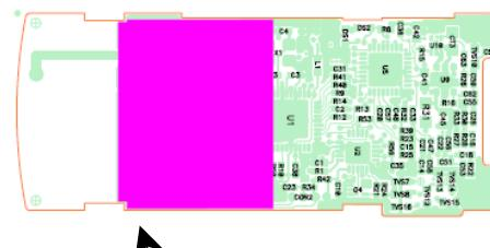
attached copper plat on this area to block the spurious radiation. when we are manufacturing this products It will be using always.
