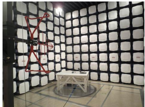
12.2 Radiated Emission 30 MHz to 1 GHz Rear View
