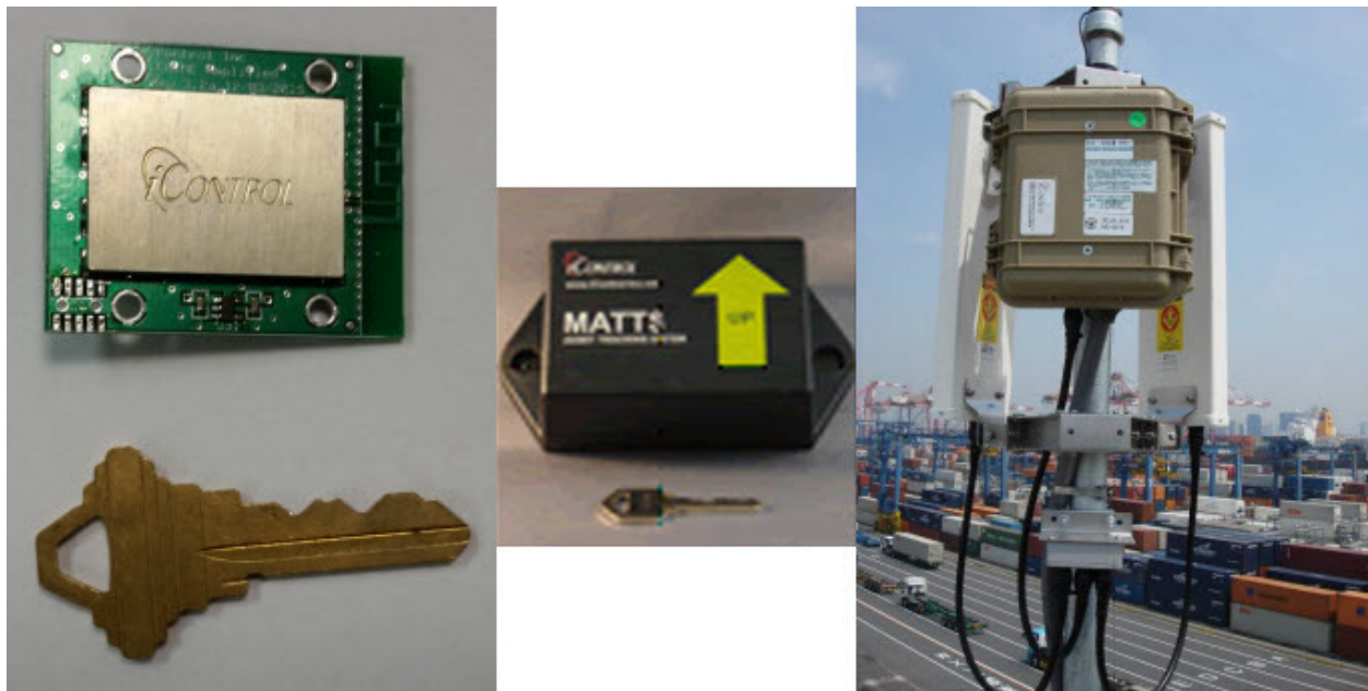
Figure 1 iCHIME™ and Network Related Devices (Left to right: iCHIME™ Module, iTAG™ repeater for iCHIME™s, iCHIME™ and iTAG™ reader)
