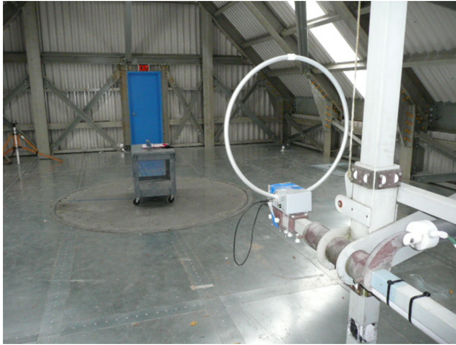
Figure 1 – Field Strength Measurement at OATS
