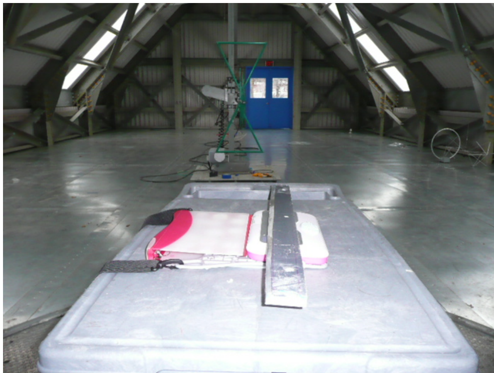
Figure 2 – Spurious Emission Measurement at OATS
