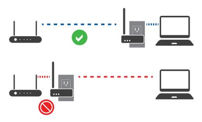
Do not place the repeater near the router or in the same room as the router.
