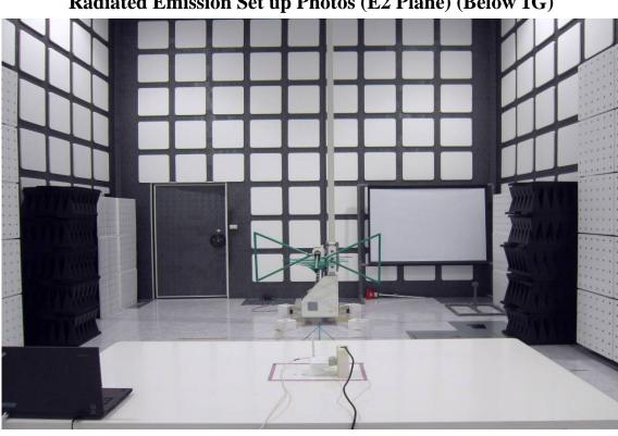
Radiated Emission Set up Photos (E2 Plane) (Below 1G)
