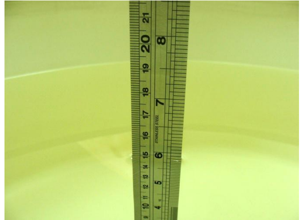
Fig 6.2 Photo of Liquid Height for Body SAR
