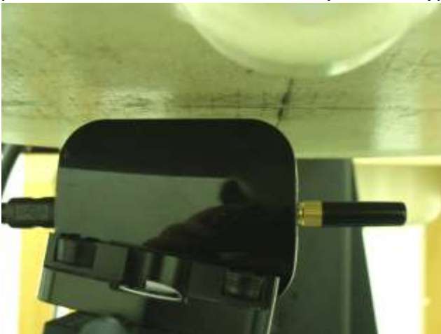
USB Configuration 4 (Vertical Back with Phantom 5 mm Gap without Clip)
