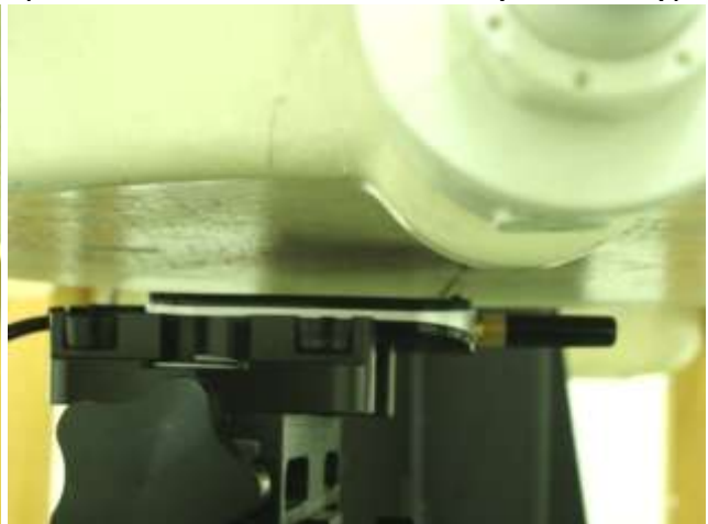
USB Configuration 1 for Back Off SAR (Horizontal Up with Phantom 10 mm Gap without Clip)
