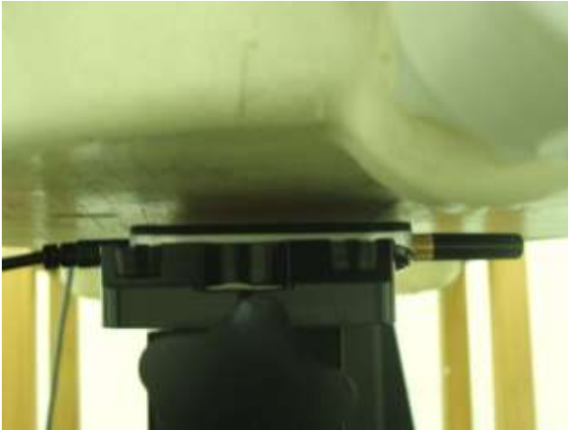
USB Configuration 2 (Horizontal Down with Phantom 5 mm Gap without Clip)
