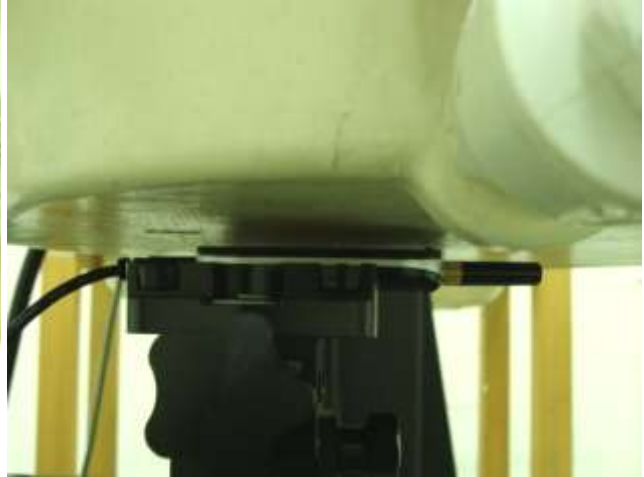
USB Configuration 1 (Horizontal Up with Phantom 5 mm Gap without Clip)
