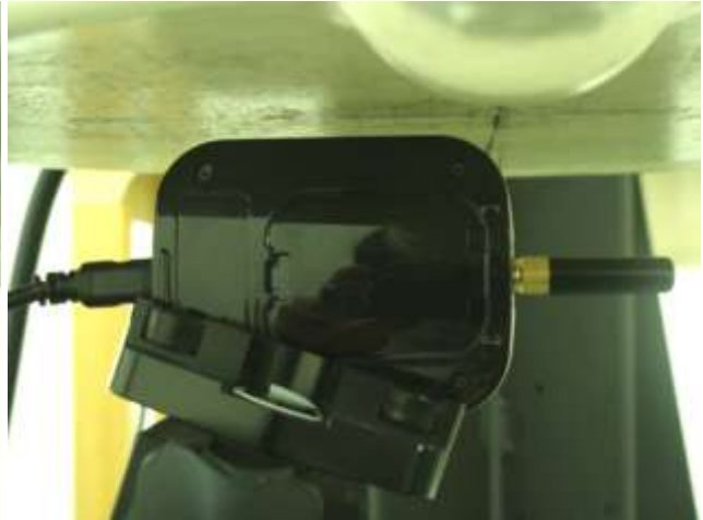
USB Configuration 3 (Vertical Front with Phantom 5 mm Gap without Clip)
