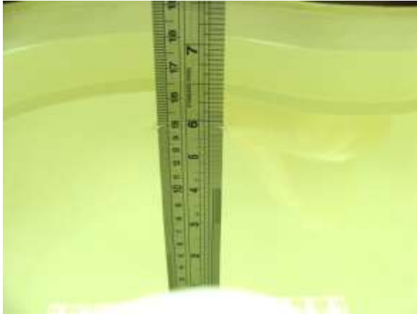
Fig 6.1 Photo of Liquid Height for Head SAR
