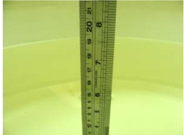
Fig 6.2 Photo of Liquid Height for Body SAR
