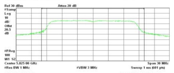
Channel Power 17.40 dBm /20.0000 MHz Power Spectral Density
