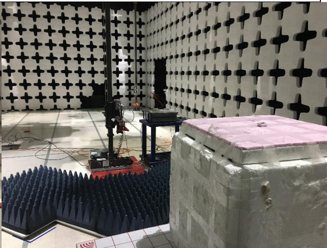
Radiated Emissions (>1GHz) – Rear View
