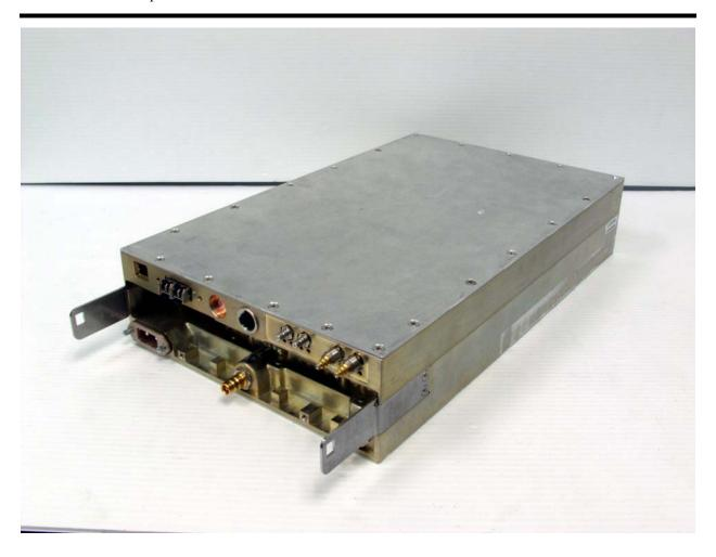
Figure E7 URM External Front View, Fan Module Removed
