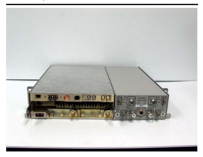
Figure E2 URM/DDM External Front View, Fan Module Removed
