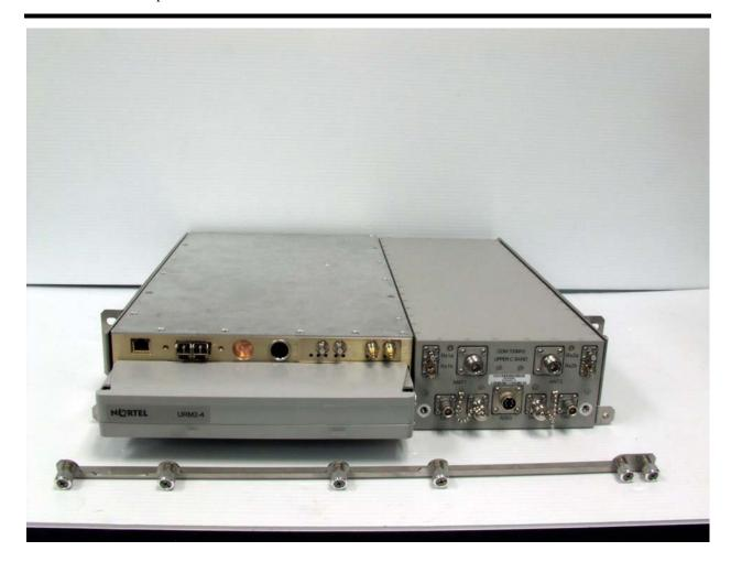
Figure E1 URM/DDM External Front View, Tray Mounted
