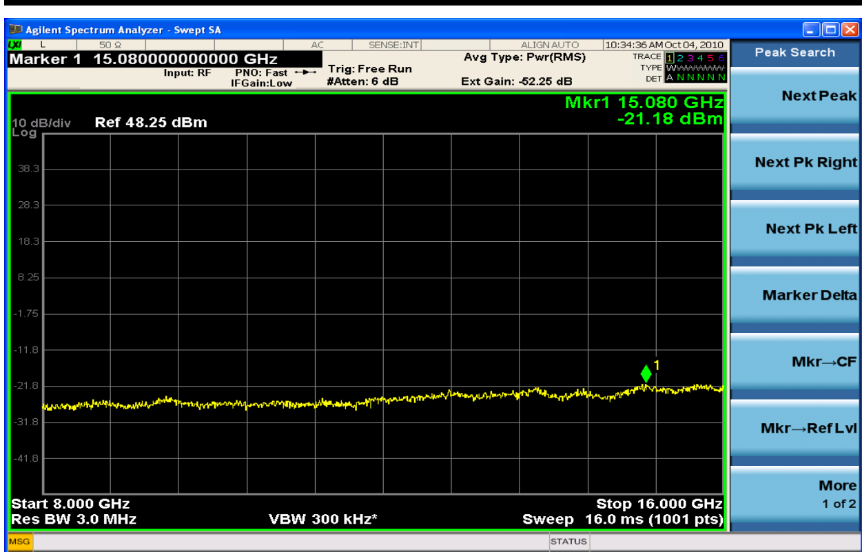
Figure 6-132 Spurious Emission TX1 64QAM 2112.5MHz - 5MHz (8GHz- 16GHz)
