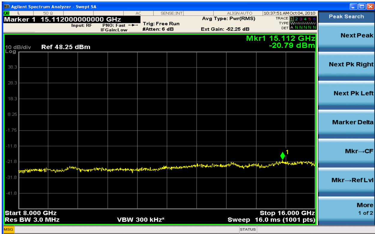
Figure 6-134 Spurious Emission TX2 64QAM 2112.5MHz - 5MHz (8GHz- 16GHz)
