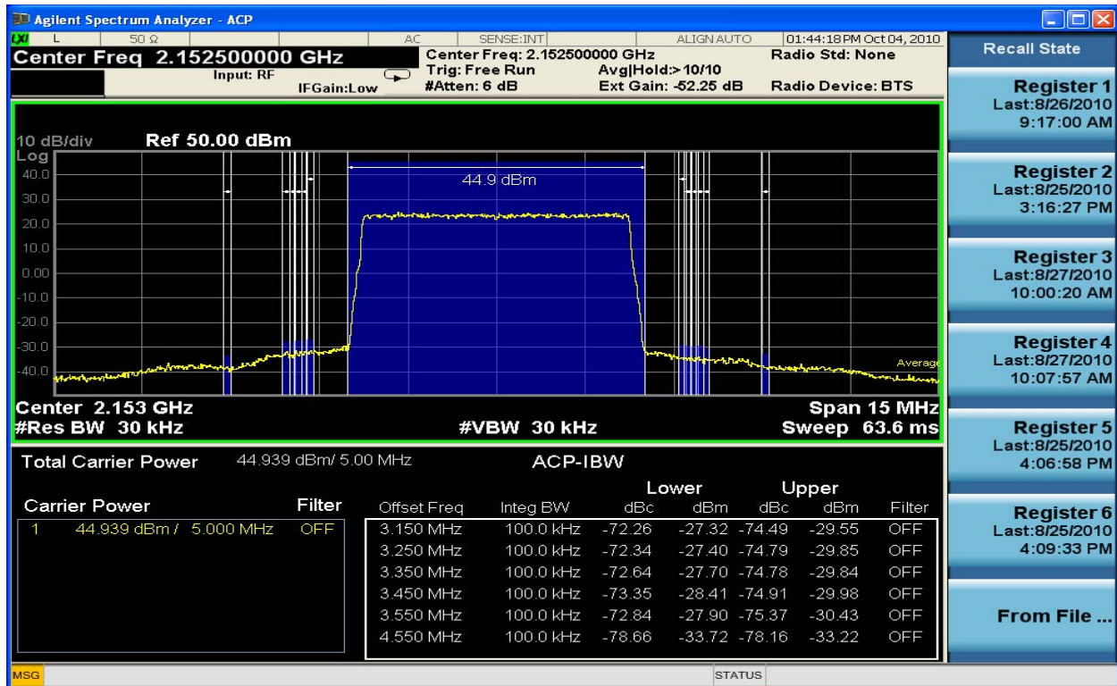
Figure 6-119 Spurious Emissions 2152.5MHz TX2_16QAM 5MHz Band Edge (ACP 650kHz – 2MHz)
