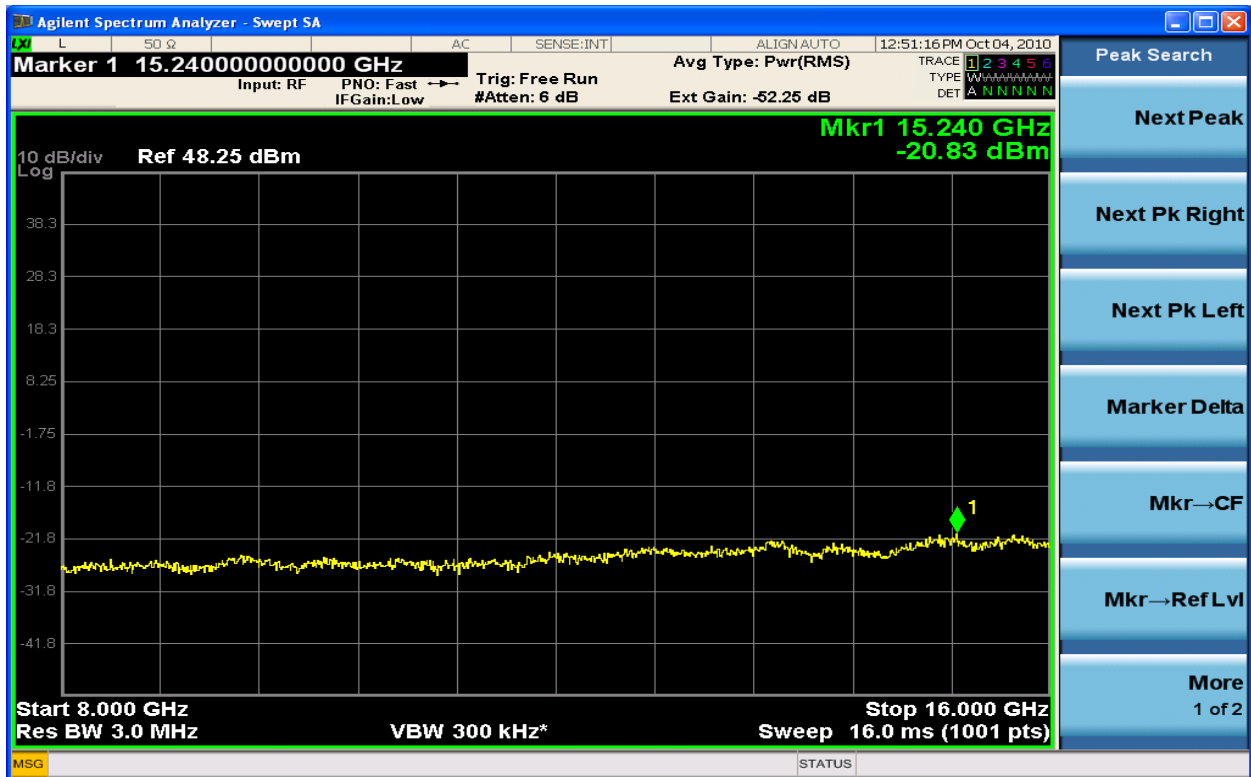
Figure 6-133 Spurious Emission TX1 64QAM 2152.5MHz - 5MHz (8GHz- 16GHz)
