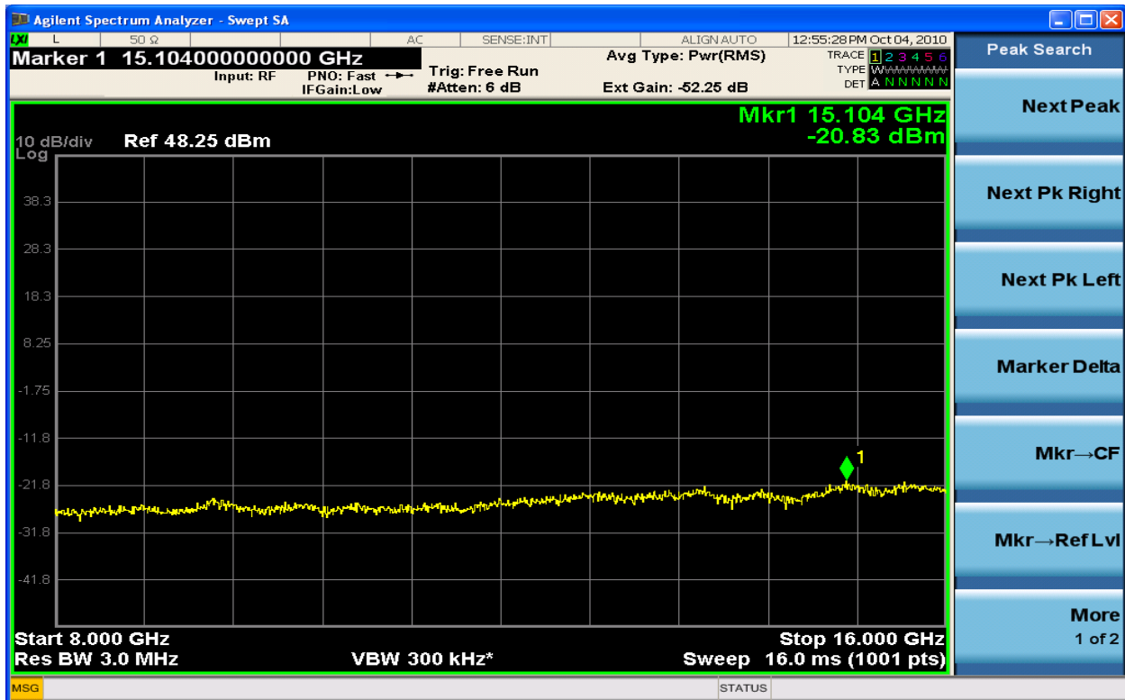
Figure 6-135 Spurious Emission TX2 64QAM 2152.5MHz - 5MHz (8GHz- 16GHz)
