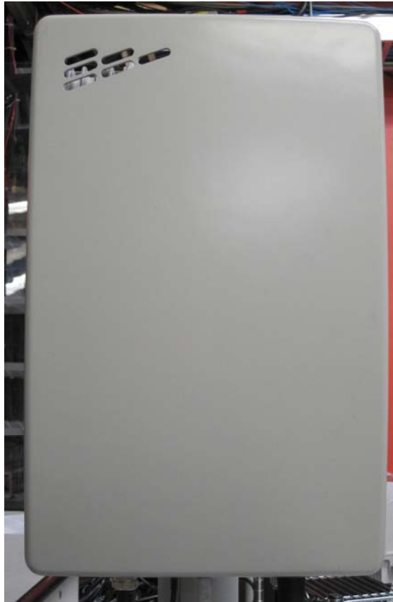
Figure 1: RRUL Front View (with Solar Shields)
