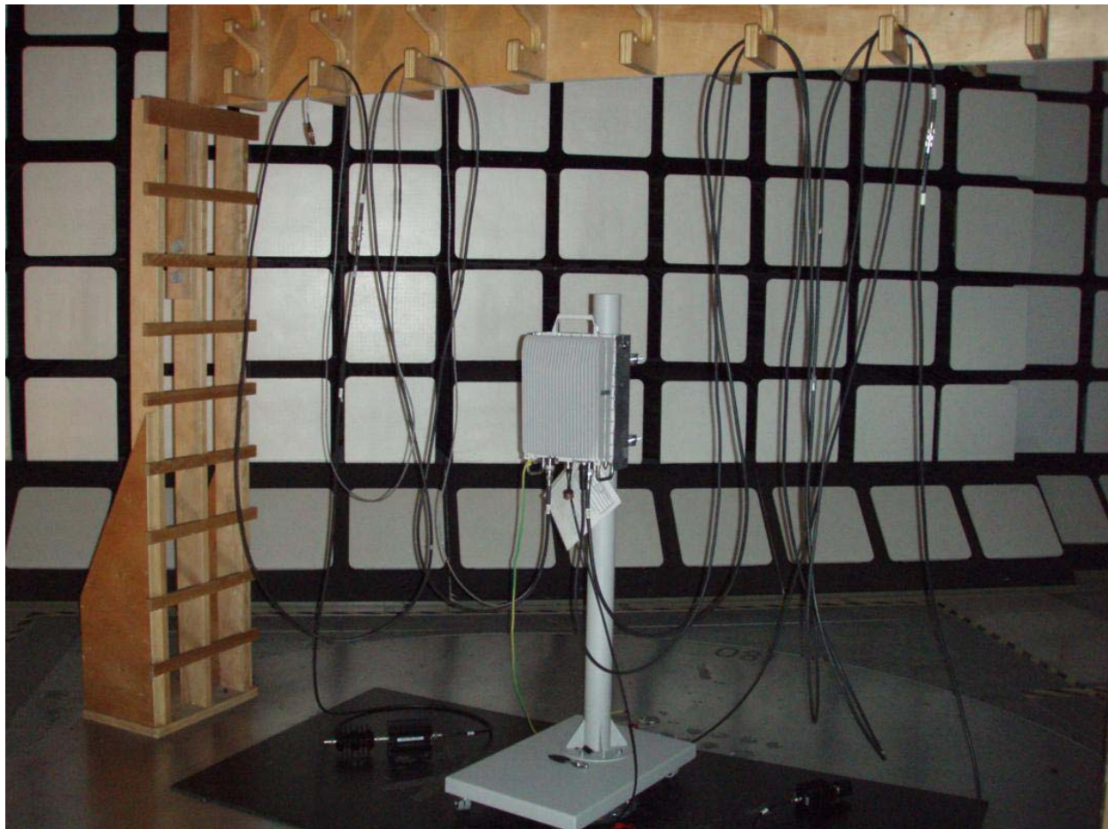
Figure 6-210 Radiated Emissions Set Up Photo
