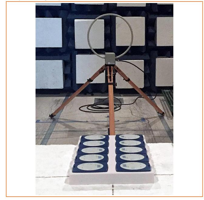
Test setup, Field Strength & Spurious Emsiions under 30MHz
