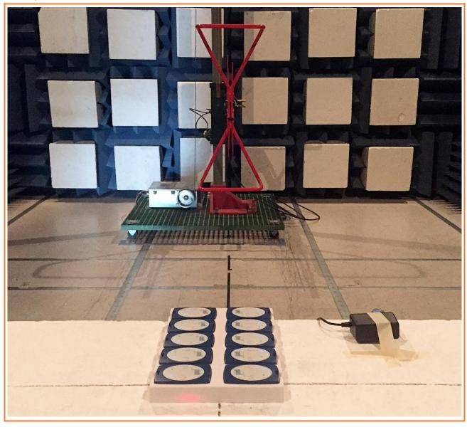
Test setup, Radiated Emissions\_PreScan, 30 to 1000MHz
