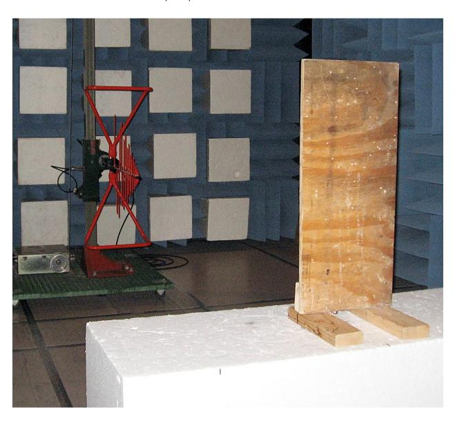
3. Test for Radiated Emissions with SAS-572, 1-6GHz
