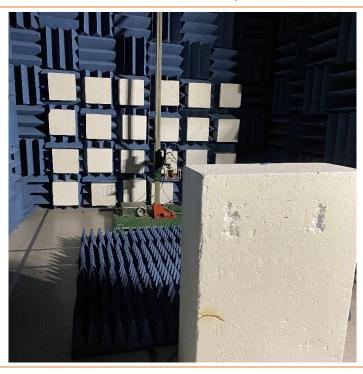
Radiated Emission 18 to 26 GHz, with SAS-572 Antenna
