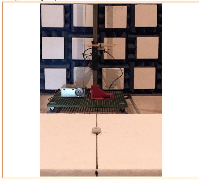
Test setup, Spurious Emissions, 1 to 5GHz
