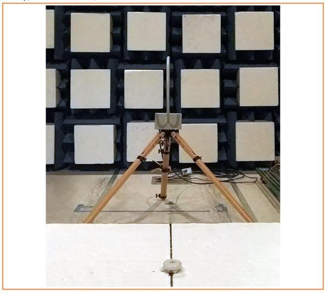
Test setup, Radiated Emissions, 30 to 1,000MHz
