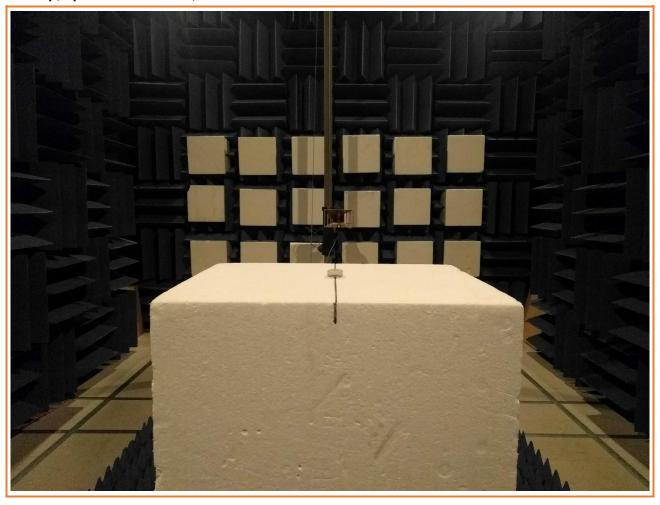
Test setup, Radiated Emissions, 30kHz to 30MHz
