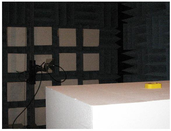
3. Tested with AL-130 for below 30MHz, Loop Antenna as followed by ANSI C63.4, Table 2
