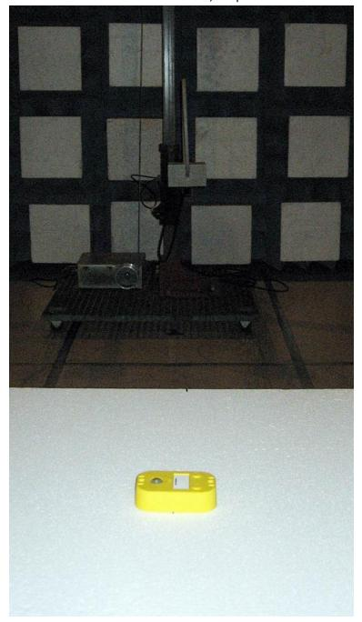
5. EUT Set up, Orthogonal X
