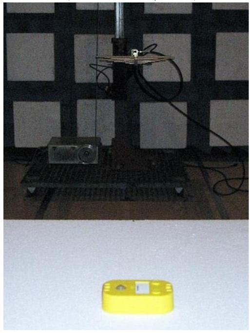
2. Tested with SAS-571 for over 1GHz, Double-ridged Guided Horn Antenna as followed by ANSI C63.10, Table 1
