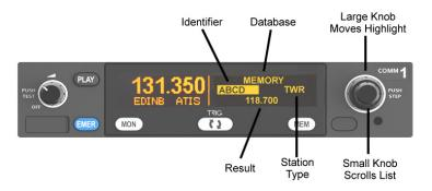
Airfield or facility identifiers are in alphabetical order. Scroll through the identifiers until you find the one that you want. Move the cursor using the large knob to highlight the station type, for example GND, TWR or APP. Pressing the MEM button at any time puts the currently selected result into the standby frequency and returns to the normal operating screen. Pressing the
