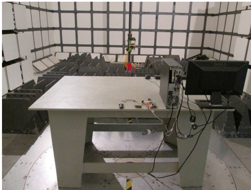
Radiated Emissions – Rear View (1-25 GHz)
