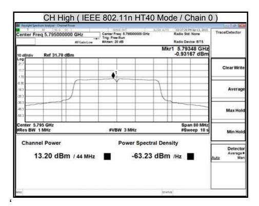
Test Mode: IEEE 802.11n HT 40 MHz mode / 5150 ~ 5250MHz
