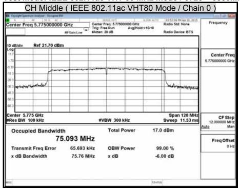
Test Mode: IEEE 802.11ac VHT 80 MHz mode / 5725 ~ 5850MHz
