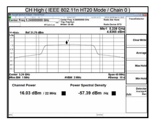
Test Mode: IEEE 802.11n HT 20 MHz mode / 5725 ~ 5850MHz
