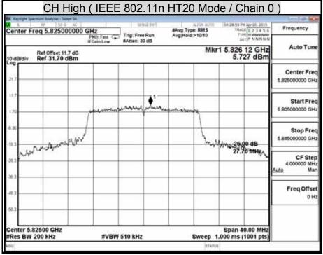
Test Mode: IEEE 802.11n HT 20 MHz mode / 5150 ~ 5250MHz
