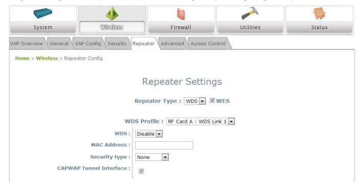
To extend the wireless coverage, EAP705 supports up to 4 WDS links for connecting wirelessly to other WDS-capable APs, or peer APs. By default, all WDS profiles are disabled.
