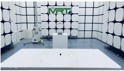
Description: Radiated Emission Test Setup for Below 30MHz-1GHz
