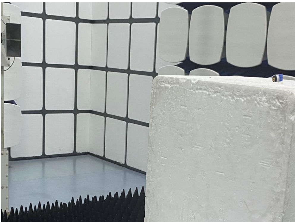
Description: Zoom for Radiated Emissions Test Setup for Above 1GHz
