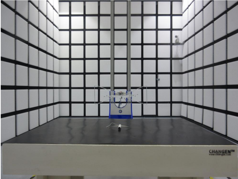
Radiated Emission Test below 1GHz
