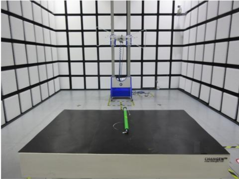
Radiated emission test below 1GHz
