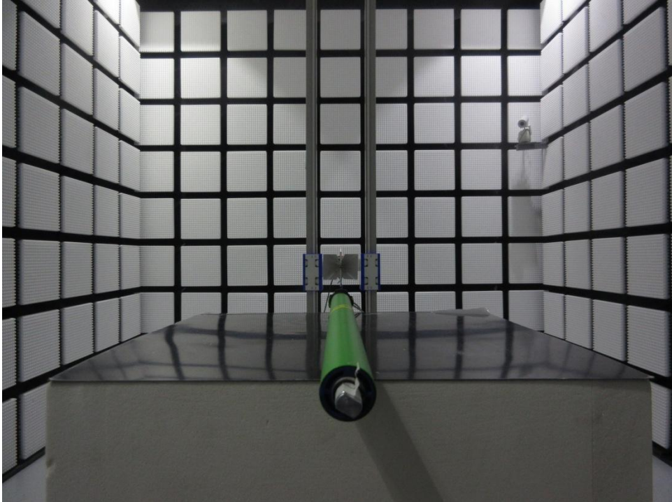
Radiated emission test above 1GHz
