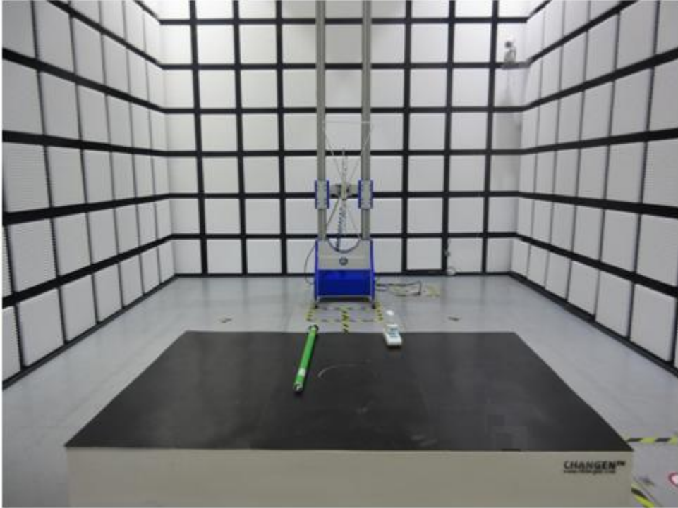
Radiated emission test below 1GHz
