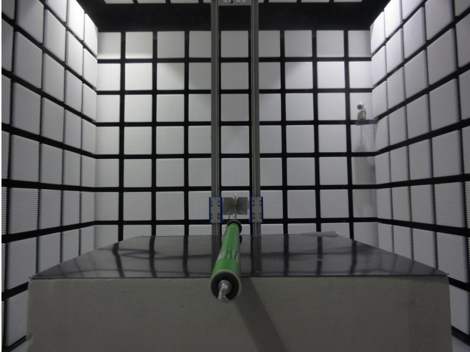
Radiated emission test above 1GHz
