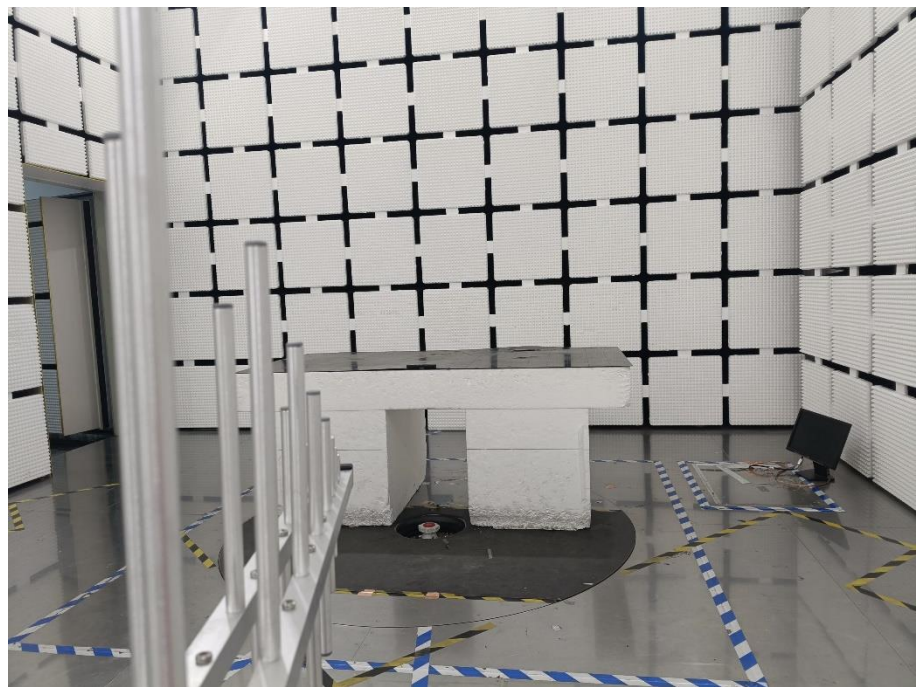
Radiation Emission Test Setup (30MHz to 1GHz)
