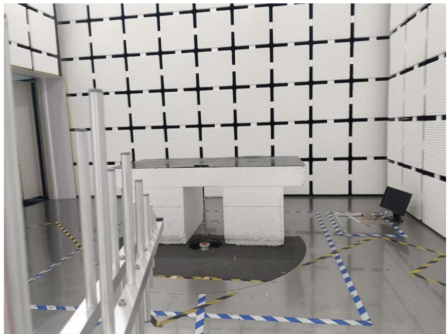
Radiation Emission Test Setup (30MHz to 1GHz)
