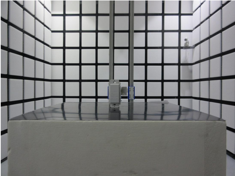
Radiated Emission Test above 1GHz:
