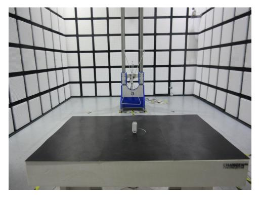
Radiated Emission Test above 1GHz:
