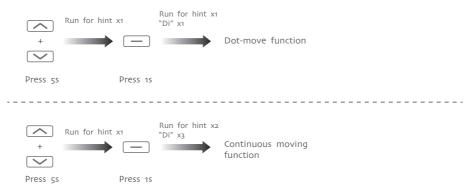
Notes: Repetitive operation dot-move and continuous moving function switching cycle, under the dot-move function, according to the upor down button more than 2S release motor linkage operation.
