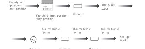
@Long press the stop button for 2s,the roller blinds will move to the third limit
