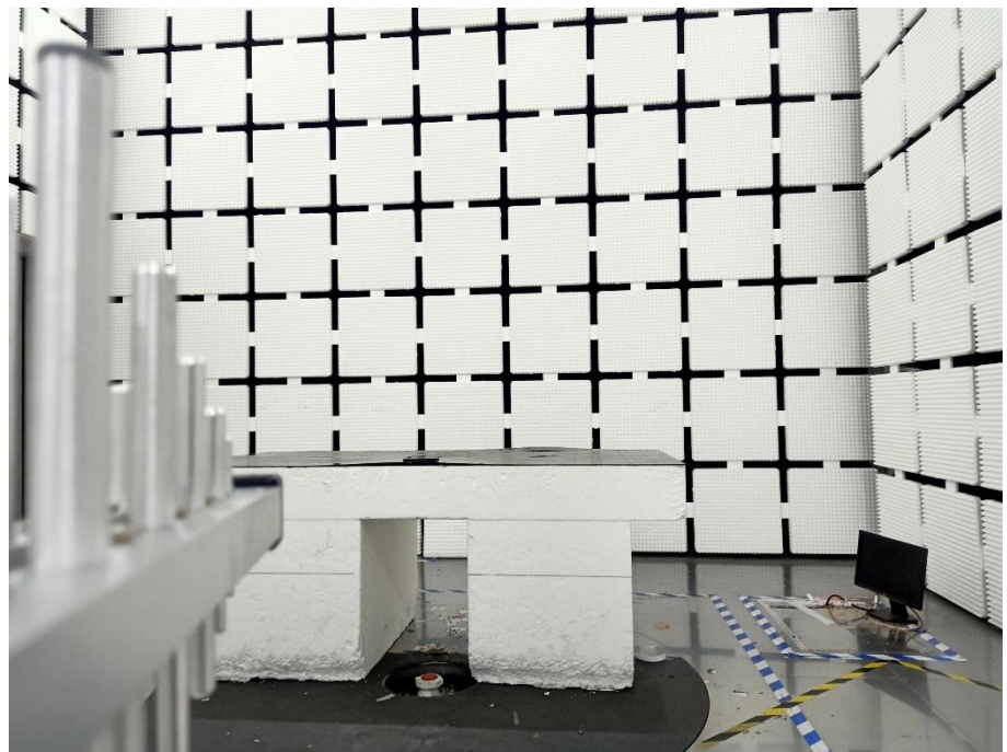
Radiation Emission Test Setup (30MHz to 1GHz)
