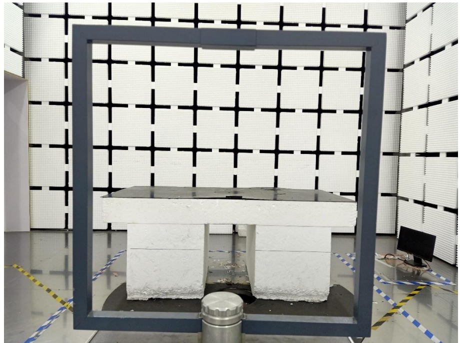
Radiation Emission Test Setup (Below 30MHz)
