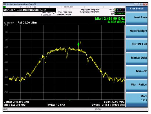
**802.11g TEST RESULT**TEST PLOT OF SPECTRAL DENSITY FOR LOW CHANNEL
